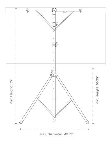
Solo Go is a portable display stand for the Solo family of screens. It comes with a black zippered soft bag(for Solo screens up to 100") with carrying handles for easy portability.
