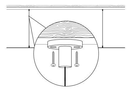
Peed the cable through the griplock leaving sufficient slack to attach the griplock assembly to the channel nuts in the upper frame. Height adjustment and leveling is done by pulling the cable through the griplock, to lower the flown height, lift the screen up to release tenson and depressing the griplock release.
