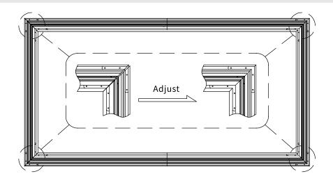
Critical Step: Frame squareness is critically important, refer to the diagram and measure the frame diagonals and compare. If the distance is not within 1/8", push from either side of the longer diagonal until each diagonal is measured within 1/8".
