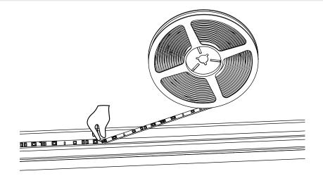
Press the lights into the channel on the frame. It is necessary to remove the adhesive backer, the LED strips are securely captured in the LED channel. LED foam must be used when rounding the corners to protect the circuit. Failure to do so will damage the LED strips. The strip should gently round the corner.
