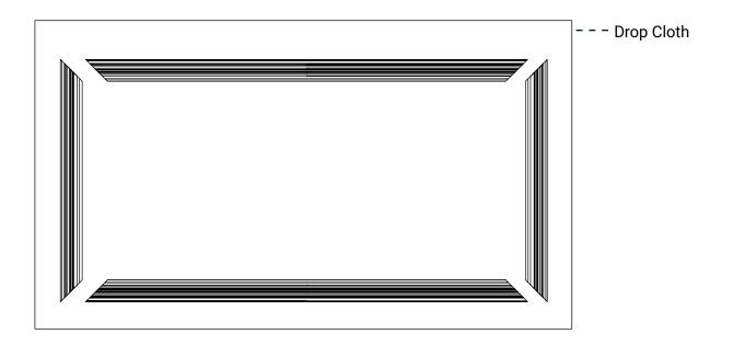
Insert the corner brackets as shown in the diagram, both thin and thick corner brackets have the same profile but as implied, one is thinner than the other. The thinner bracket is used in the channel closest to the outer frame edge.
