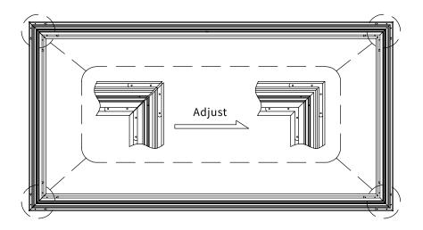
Critical Step: Frame squareness is critically importance, refer to the diagram and measure the frame diagonals and compare. If the distance is not within 1/8", push from either side of the longer diagonal until each diagonal is measured within 1/8".
