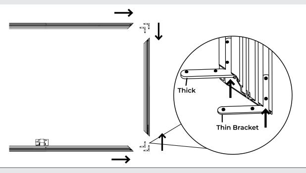
Align the edges to ensure they are at a right angle. With the included allen wrench lightly tighten two of the set screws to lock in the corners.
