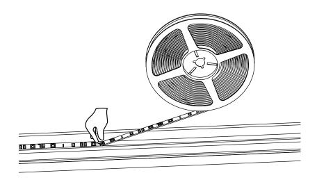
Press the lights into the channel on the frame. LED foam must be used when rounding the corners to protect the circuit. Failure to do so will damage the LED strips. The strip should gently round the corner.
