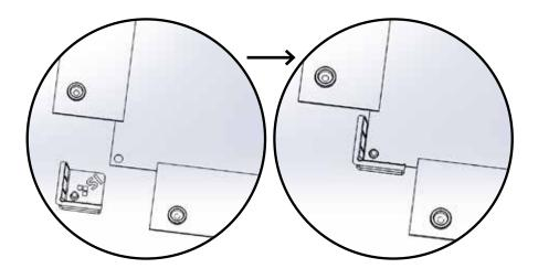
Then check to make sure the screen material is flat and adjust the snap positions if necessary to flatten the screen material. Once all snaps are attached flip screen over and make sure that the screen material is flat and tight everywhere.
