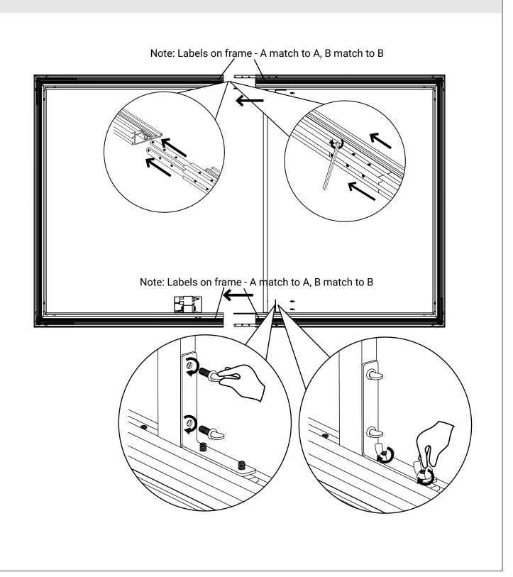
Align the edges to ensure they are at a right angle. Finger-tighten two of the set screws to lock in the corners.
