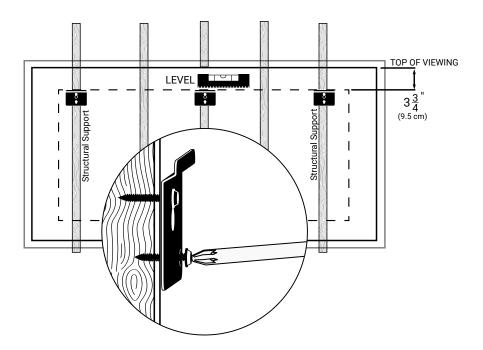
2 Use two or more people to carefully lift the screen up and latch onto the brackets.
