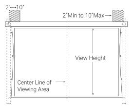
3. Securely attach the ceiling mount bracket to structural ceiling mounting surfaces with wood fasteners included.
