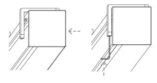
6. Use the 3/32" hex key to tighten the locking screw in the back of the brackets.
