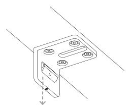
5. Hook the cassette onto the brackets. Then use the 5/64" hex key to turn the bottom screw until the cassette bottoms out on the bracket.
