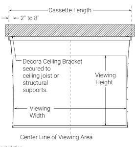
3. Attach the Décora Ceiling Brackets to the ceiling joists or other structural supports. The included screws can be used for securing to wood structural supports if securing to other materials then installer must select appropriate fasteners. Make sure brackets are plumb, and both on the same level line.
