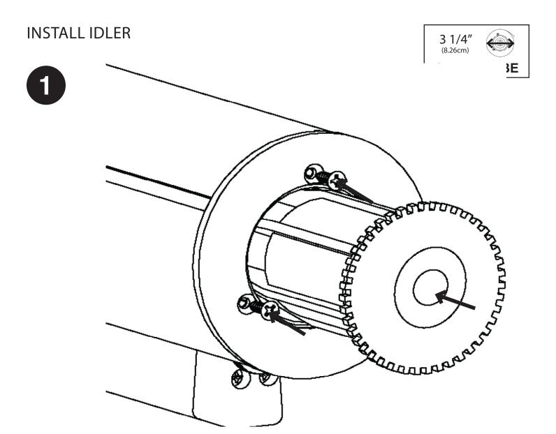
Slide the idler into the opposite end of the tube and secure with 3 phillips head screws. Make sure the idler is retracted all the way in preparation for installation into the case. Turn to page 18 to install the screen in the case.
