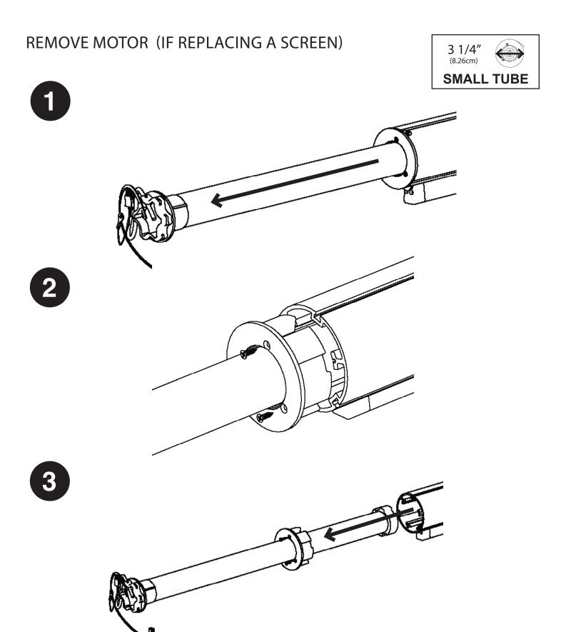
Slide the motor out to get access to the retaining screws. Remove and set aside the retaining screws, then completely remove the motor.
