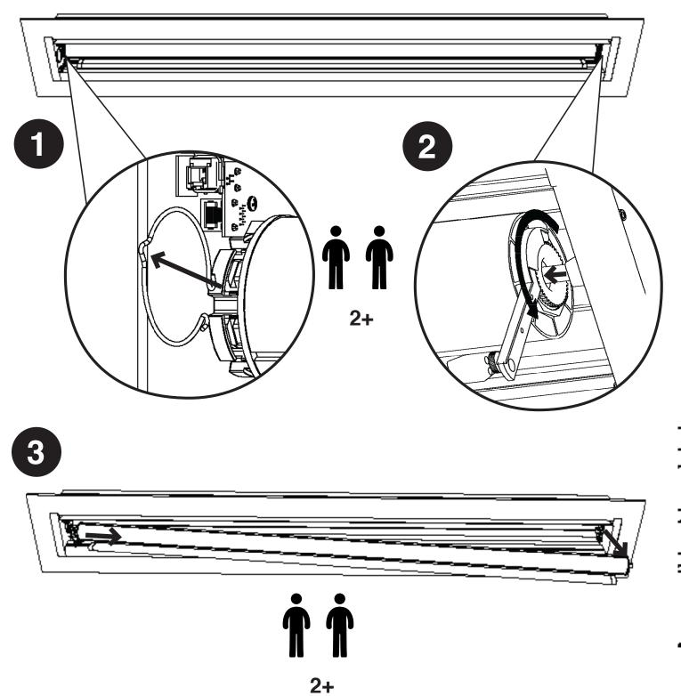
Remove the motor retaining ring from the left end of the case. Turn the teeth on the idler counterclockwise with the included tool to retract the idler. Then lower the screen asembly down and out of the case.
