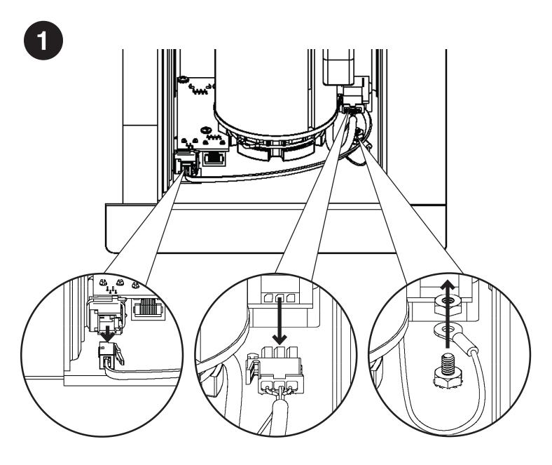
Disconnect the control, power, and grounding cables from the left side of the case. NOTE: On above ceiling applications with pigtails/hardwired you will need to access the junction box above the ceiling through the ceiling access hatch to disconnect and pull the wire through the end plate.
